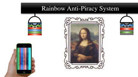
Fig. 1. Application of Rainbow : preventing mobile-camera-based piracy in museums. Our system can seriously pollute a pirated image while maintaining good visual quality for human viewers.
